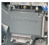
Integrated stone catcher All PT pumps feature a stone catcher protecting the pump internals from any suspended solids. The stone catcher has easy-access cleaning covers and comes with dual vacuum gauges to monitor pump performance.
